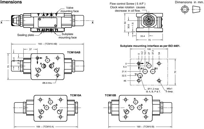
Note : Rotate the valve around horizontal axis 'X' - 'X' by 180° to convert from METER-IN control to METER-OUT control. Valve fixing S.H.C Screws are not in scope of supply. Tightening torque for S.H.C Screws is 16 Nm.
