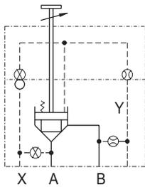
VD4S\*\*-\*D4 - 34\* with stroke limiter
