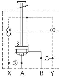
VD4S\*\*-\*23-3B\* with stroke limiter
