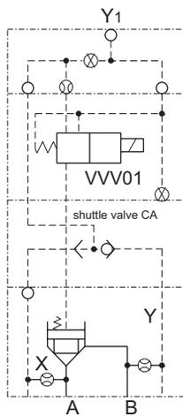
VD4S \*\*-\*C2-\*\*\*- CB } with shuttle valve CA
