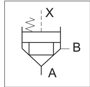
The basic element incorporated in both the body mounted and cartridge type (manifold) mounted series is the main cartridge comprising poppet spool, sleeve and spring. The wide range of optional combinations are based on an integrated system which offers easy modification to existing circuits incorporating the Veljan Seat valve/cartridge modules. Close manufacturing tolerances permit simple change or addition without special fitting.
