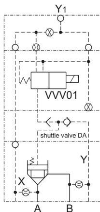
VD4S \*\*-\*C2-\*\*\*- DB } with shuttle valve DA
