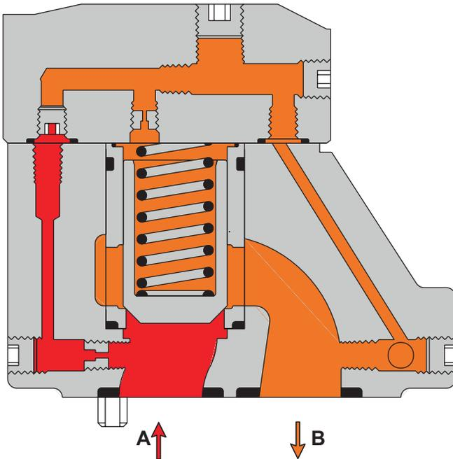
The body mounted valve series VD4S is available in 3/8", 3/4" and 1 1/2" sizes. It has application and production advantages when used in circuits on machines produced in small or medium batches. Since all pilot passages and control orifices are contained within the seat valve subplate mounted body, the manifold block on which they are mounted becomes a simple distributor block without the necessity for small drillings or close tolerances.
