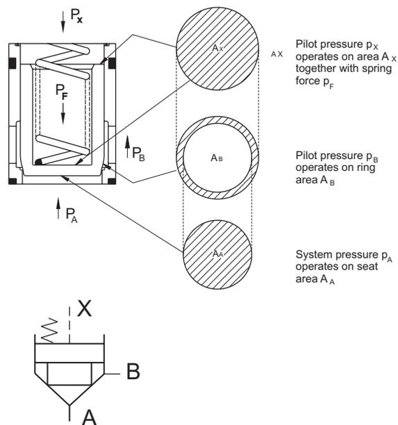
Example : With a ratio of 95% seat area to 5% ring area and a spring pressure = 2.2 bar then the following cracking pressures apply.
