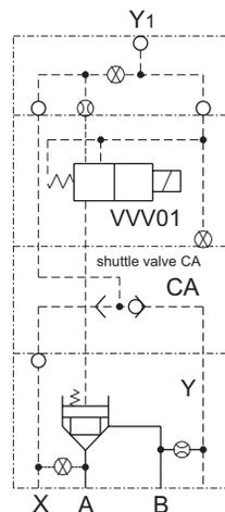
VD4S\*\*-\*D2-\*\*\*- CB } with shuttle valve CA
