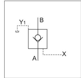
VC4V Pilot operated check valves works as a normal check valve for flow from port A to port B. Flow from port B to port A is blocked.
